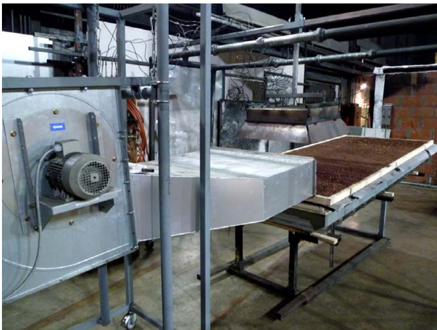
Illustration 2: The testing equipment for test procedure 3 with blower and radiant heater and a 1.2 x 3.0 m green roof build-up, initially without vegetation.
