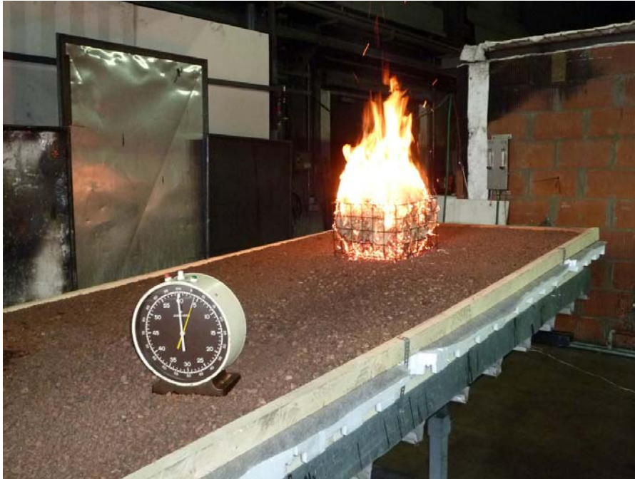
Illustration 1: First of all, a control fire test based on DIN 4102-7 was carried out in accordance with test procedure 1 of DIN EN 1187. The build-up was not affected.
