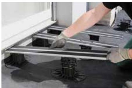
The Cantilever Arm Support allows for close connection to doors or insulating fillets. The doorstep height can be reduced to a minimum of 50 mm, if a drainage channel is used in front.
