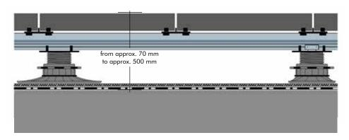
Slabs of e.g. concrete or natural stone, or ceramic or wood decking\*
