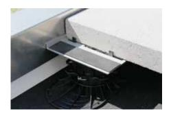
In the edge areas, the practical edge retainers ensure a stable position of the pavers without them wobbling. Thanks to the recesses in the edge retainers, the joint spacers on the support plate continue to ensure a uniform joint pattern here too.
