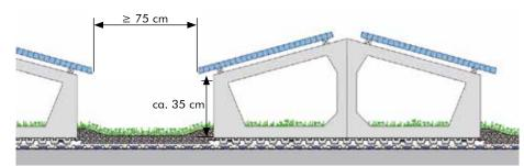
The front edge of the solar panels has a sufficient distance to the substrate surface so that plants can still grow under the panels.
