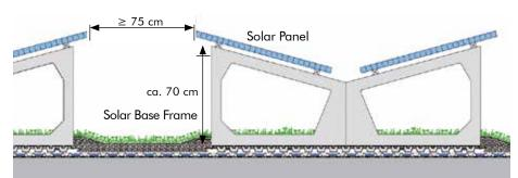
distributed from there in both directions. In this case, a rather lush vegetation can be expected under the solar panels. The plants are relatively easy to access from the walkways between the panels because the panels have their maximum distance of approx. 70 cm to the substrate surface there.
