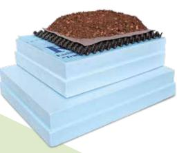
With inverted roofs, layers that prevent the diffusion of damp must not be installed above the XPS thermal insulation boards. Therefore, the water retaining protection mat must be replaced by the diffusion permitting Separation Membrane TGV 21. In the case, that root barriers are necessary they have to be placed below the insulation boards directly onto the waterproofing. A deeper substrate layer compensates for the water retention capacity of the protection mat.
