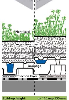
Build-up height: ca. 120 resp.150 mr Weight, saturated: ca. 105 kg/m² Water retention capacity: ca. 33 l/m² Plant level "Rockery Type Plants"
