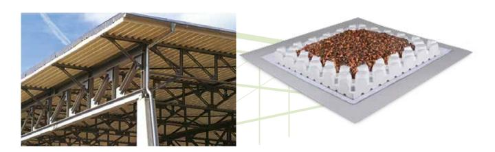
For some roof areas, even the Standard Build-up "Sedum Carpet" is too heavy. The solution is a system build-up with Floraset® FS 75. Less substrate is required as it is not applied equally but mainly fills the gaps between the high studs of the element. Although they start growing mainly in those "planting pots" the
