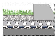
Plug Plants FB 50 "Sedum Carpet" or Sedum Cuttings System Substrate, depth depends on the superimposed load required ZinCo Solar Base® SB 200 Fixodrain® XD 20 Root Barrier WSF 40, if waterproofing is not root-resistant
