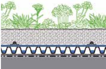
System Build-up "Urban Climate Roof" System Build-up with maximum evaporation capacity
