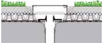
System Build-up "Stormwater Management Roof" Stormwater retention with a green roof
