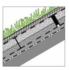
Build-up height: ca. 120 mm ca. 155 kg/m<sup>2</sup> Weight, saturated: Water retention capacity: ca. 64 l/m<sup>2</sup>
