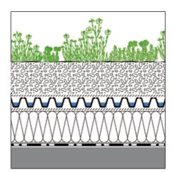
Build-up height: from ca. 110 mm Weight, saturated: from ca. 120 kg/m²
