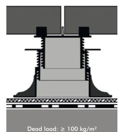
Slabs of concrete, natural stone, d ≥ 40 mm or wooden surfaces
