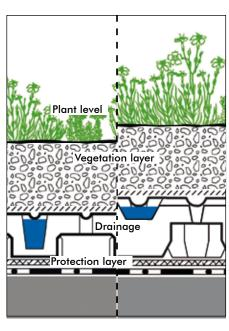
Build-up height: ca. 120 resp.150 mm Weight, saturated: ca. 105 kg/m<sup>2</sup> Water retention capacity: ca. 33 l/m<sup>2</sup>
