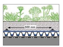
Build-up height: from 140 mm\* from 155 kg/m<sup>2</sup> Weight, saturated: Water retention capacity: from 51 l/m<sup>2</sup> **Evaporation capacity:** 7-10 mm/d
