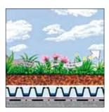
Green Roof vegetation helps to filter out dust and smog particles. Nitrates and other harmful materials are absorbed by the plants out of the air and rainfall and bound within the substrate.
