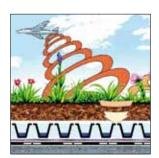
Planted areas are natural sound insulators and absorb more sound than hard surfaces. Green Roofs reduce reflective sound by up to 3 dB and improve sound insulation by up to 8 dB. This is very effective for buildings near airports, noisy nightclubs and factories.
