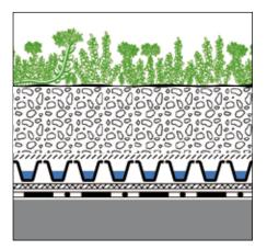
Build-up height: from ca. 90 mm Weight, saturated: from ca. 95 kg/m<sup>2</sup> Water retention capacity: from ca. 25 l/m<sup>2</sup>
