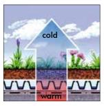
A Green Roof has the ability to buffer temperature extremes and improve the buildings energy performance.
