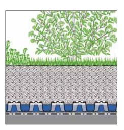
Build-up height: from 270 mm from 370 kg/m<sup>2</sup> Weight, saturated: Water retention capacity: from 136 l/m<sup>2</sup>
