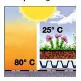
A Green Roof protects the waterproofing from climate extremes, UV exposure and mechanical damage.
