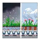
A Green Roof can reduce water run-off by 50–90%; any water flows from the roof with a delay.
