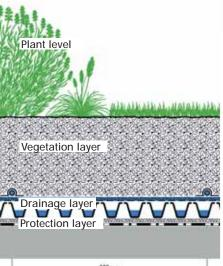
Build-up height: from 200 mm Weight, saturated: from 230 kg/m² Water retention capacity: from 80 l/m²
