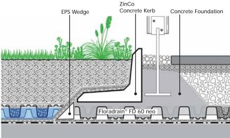
The complete drainage area remains intact when the foundation is built as a strip foundation. For dam up area (left), the waterproofing is drawn upwards so that water cannot enter the walkway build-up (right).
