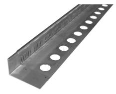
Heavy-duty angle profile made of stainless steel with drainage slots and perforation in the support leg for fixation onto the waterproofing.
