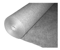
Geotextile of needled and thermally strengthened polypropylene, applicable as filter sheet above drainage elements for normal mechanical stress.
