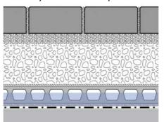
Paving slabs in a bedding of stone chippings
