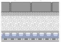
Paving slabs in a bedding of stone chippings
