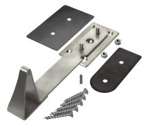
Stable shear retainer, made of solid stainless steel, to be installed on sealed pitched roofs as loose flange / fixed flange construction. Replaces wooden shear barriers in connection with ZinCo eaves profiles.
