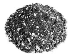
Growing Medium for Semi-intensive green roofs in multiple layer build-up.
