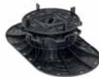
Elefeet® E 60 adjustable from 60–106 mm
